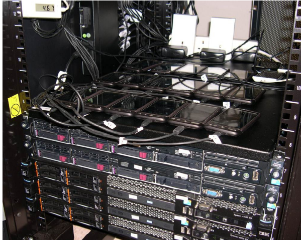
Figure 1: Subset of the SmartLab smartphone fleet connected locally to our datacenter. More devices are connected over the wireless and wired network.
