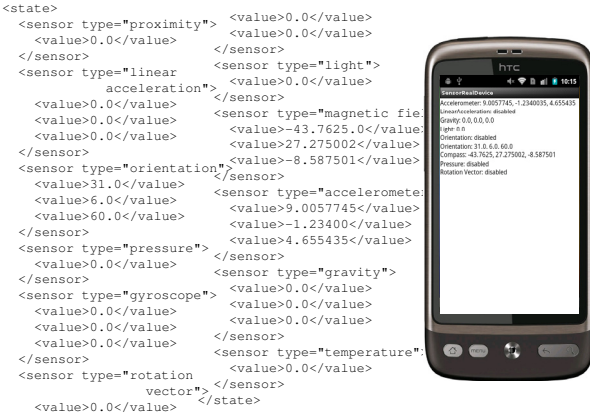
Figure 13: Sensor/GPS Mockup (RM): (left, center) A data trace of various sensor measurements encoded in XML. The given file can be loaded to ARDs and AVDs through this subsystem; (right) An application built with SLSensorManager using the measurements.
